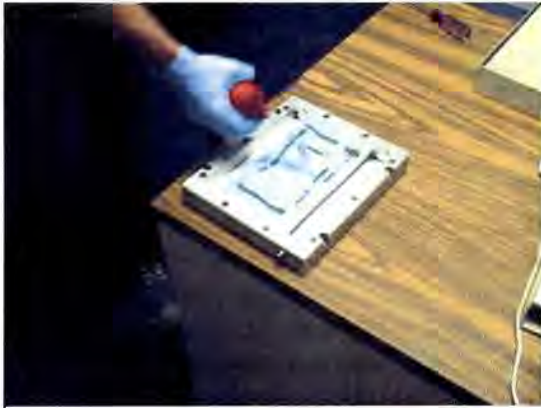
Figure 23– Applying Motor Oil to Filter
